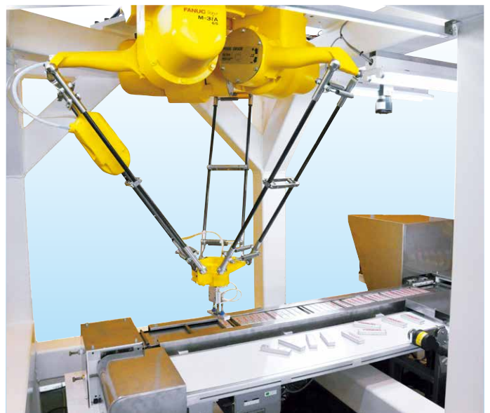
High speed arranging the foods by M-3iA/6S
